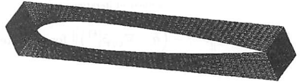
Fig. 4 Triangular element (8,192 elements)
