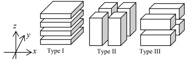
Fig.5 Illustration of three type of domain decomposition
