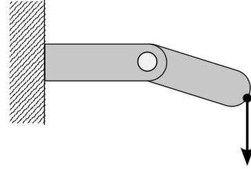
(b) Link mechanism under bending load.
