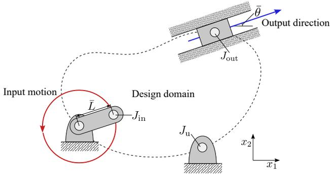
(a) Problem definition to synthesize a linkage mechanism.
