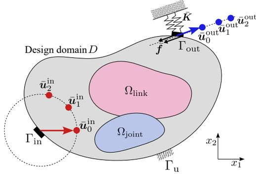
(b) Design domain for topology optimization of a linkage mechanism.
