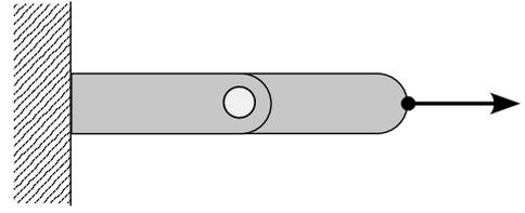
(a) Link mechanism under tensile load.
