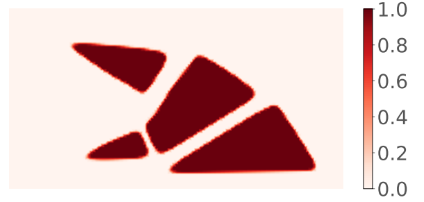
Fig. 8: The regions G(p) that violate the molding constraint when the constraint is not considered.
