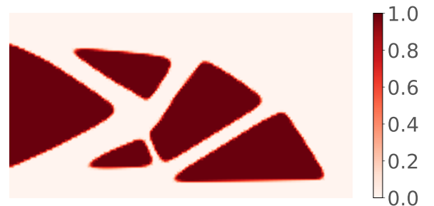
Fig. 15: The regions G(p) that violate the molding constraint when the constraint is not considered.
