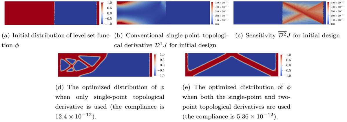
Fig. 6 Initial design, topological derivatives and optimized designs for condition 1.
