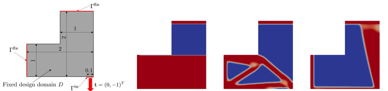
(a) Domain and boundary conditions. (b) Initial distribution of level set function  $\phi$ . (c) The optimized distribution of  $\phi$  when only single-point topological derivative is used (the compliance is  $4.0 \times 10^{-12}$ ). (d) The optimized distribution of  $\phi$  when both the single-point and two-point topological derivatives are used (the compliance is  $3.8 \times 10^{-13}$ ).
