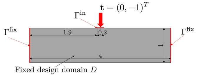
Fig. 5 Domain and boundary conditions for condition 1.
