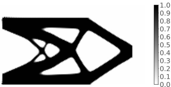
Fig. 8: The structure domain ( $\mathcal{H}(\phi, \epsilon_u)$ ) without overhang constraint after 500 steps.
