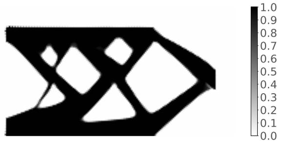
Fig. 10: The structure domain ( $\mathcal{H}(\phi, \epsilon_u)$ ) with overhang constraint after 500 steps.
