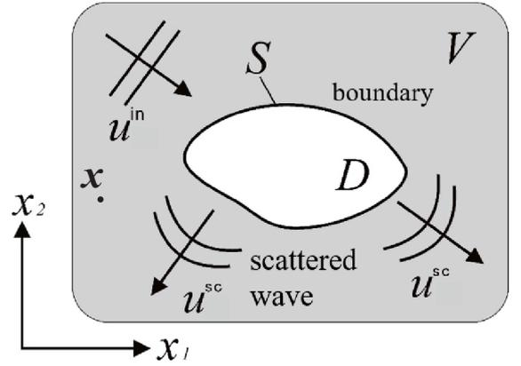
Fig. 1 Elastic wave scattering by a traction free cavity in an anisotropic viscoelastic solid.
