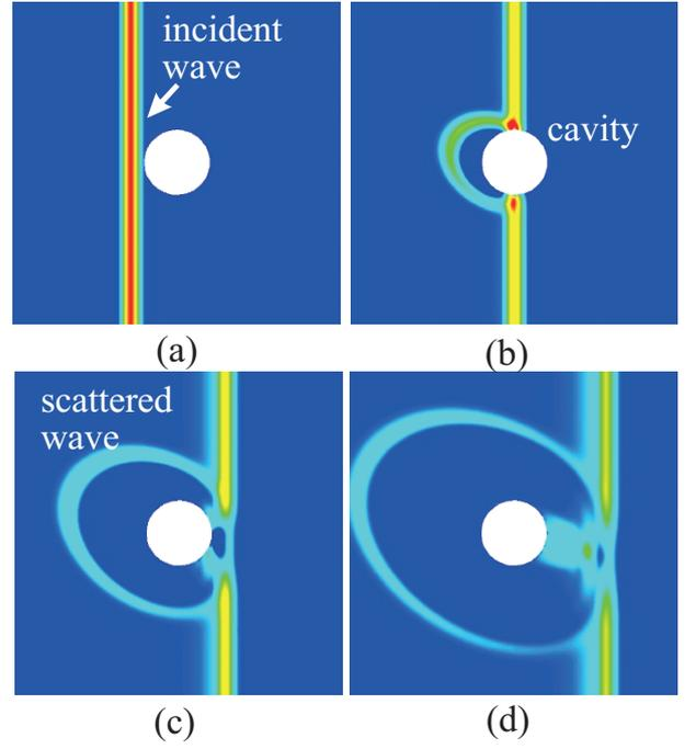
Fig. 8 Total wave fields  $|u|/u_0$  around a cavity in the graphite-epoxy with the initial elastic constant  $C_{\alpha\beta}^0/C_{66}^0$  given in Eq.(22).
