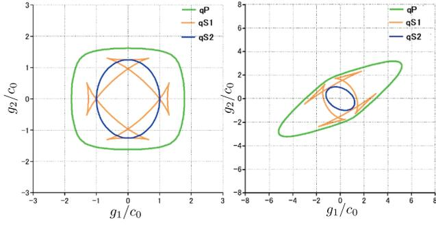
Fig. 5 Group velocity curves for (a) austenite steel (b) graphite-epoxy with 30° inclined anisotropic principle axis.
