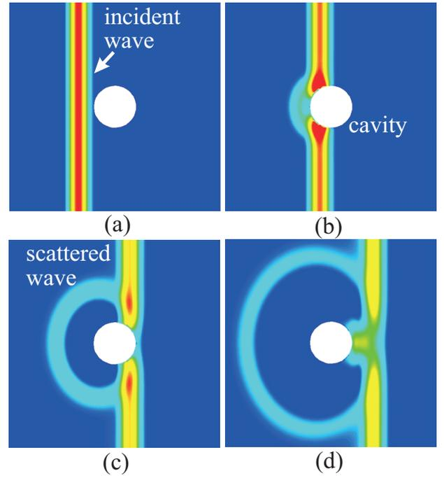
Fig. 6 Total wave fields  $|u|/u_0$  around a cavity in the austenite steel with the initial elastic constant  $C_{\alpha\beta}^0/C_{66}^0$  given in Eq.(21).
