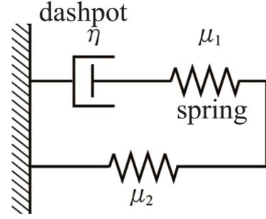
Fig.2 Standard linear solid model for viscoelasticity.
