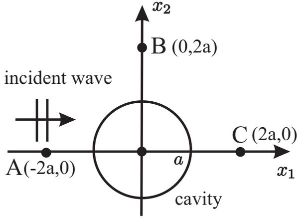
Fig. 3 Elastic wave scattering by a cavity with radius  $a$  in an anisotropic viscoelastic solid.
