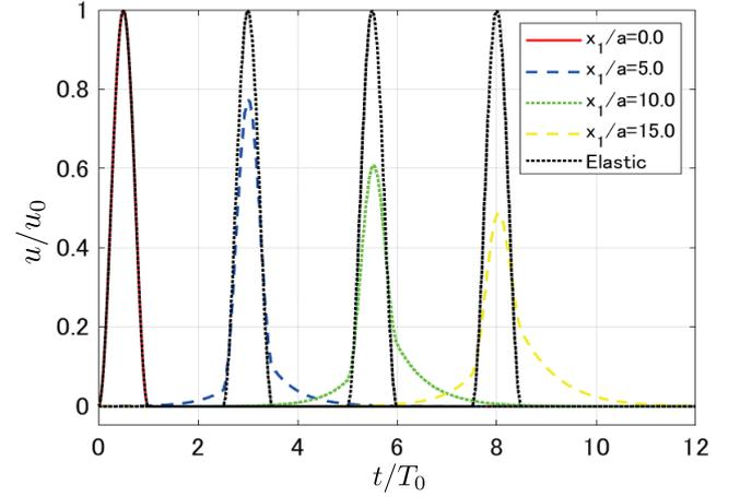
Fig. 4 Time variation of the incident plane wave at  $x_1/a = 0.0, 5.0, 10.0, 15.0$ .
