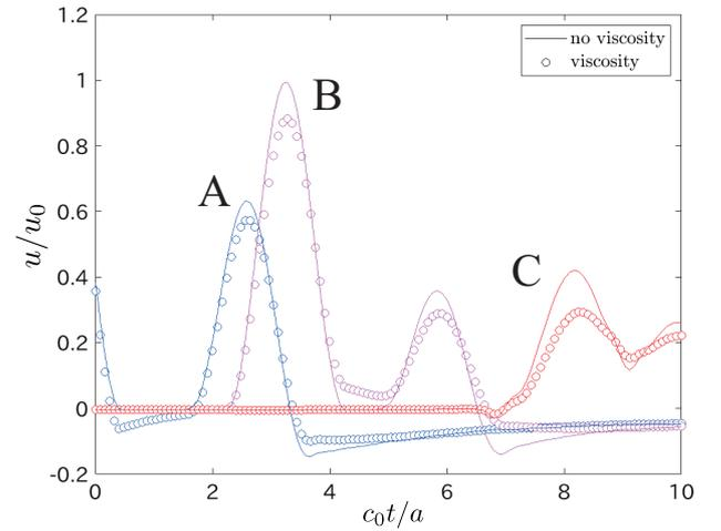
Fig. 9 Total displacement A, B, and C in graphite-epoxy with the initial elastic constant  $C_{\alpha\beta}^0/C_{66}^0$  given in Eq.(22).
