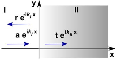
Fig. 10: We have shown the transmission and reflection at the stealth region interface. Here,  $k_I$  and  $k_{II}$  are the corresponding wavevectors in the regions I and II, respectively. Here,  $a$ ,  $r$  and  $t$  are the incident, reflected and transmitted amplitudes, respectively.
