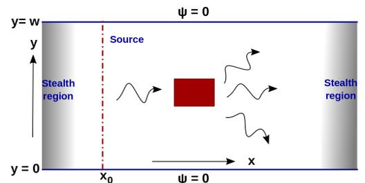
Fig. 5: We show a schematic picture of scattering in a 2D waveguide of width  $w$ . We place the stealth region at either end of the waveguide. The wave propagation is along the  $x$ -axis.
