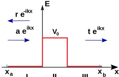
Fig. 1: Scattering through a 1D barrier of height  $V_0$ . We consider an incoming plan wave with an amplitude  $a$  and the energy  $E$ . The corresponding wavevector is  $k = \sqrt{2m^*E/\hbar^2}$ . Here,  $r$  and  $t$  are the reflection and transmission amplitudes, respectively.
