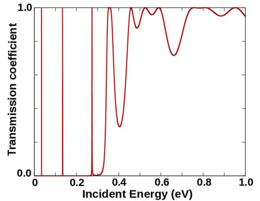
Fig. 4: We have plotted the transmission coefficient as a function of energy for a double barrier potential. Each of the barriers is of height 0.3eV with a width of 100Å and are 100Å apart.
