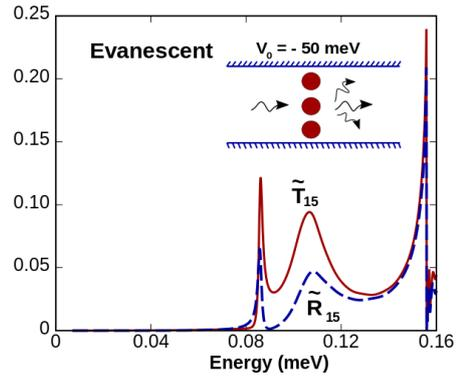
Fig. 9: The transmission ( $\tilde{T}_{15}$ ) and reflection ( $\tilde{R}_{15}$ ) coefficients are shown as a function of energy for the evanescent mode  $n = 5$ , with an incoming wave from the mode 1 at a distance  $l = 50\text{\AA}$ , for scattering through vertically aligned three circular holes of radius  $30\text{\AA}$  whose centers are  $100\text{\AA}$  apart, and depth  $-50\text{ meV}$ .
