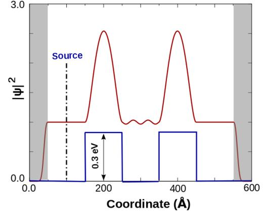
Fig. 3: Probability distribution for the first above-barrier resonant state with incoming energy 0.355eV is shown. The source is located at 100 Å. The stealth region is shaded in gray and the width of the stealth region is equal to 50 Å.
