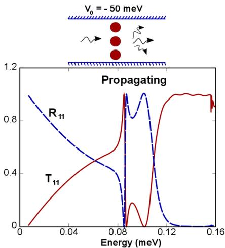
Fig. 8: The transmission ( $T_{11}$ ) and reflection ( $R_{11}$ ) coefficients are shown as a function of energy for the propagating mode  $n = 1$ , with an incoming wave from the same mode for scattering through vertically aligned three circular holes of radius  $30\text{\AA}$  whose centers are  $100\text{\AA}$  apart, and depth  $-50\text{ meV}$ .
