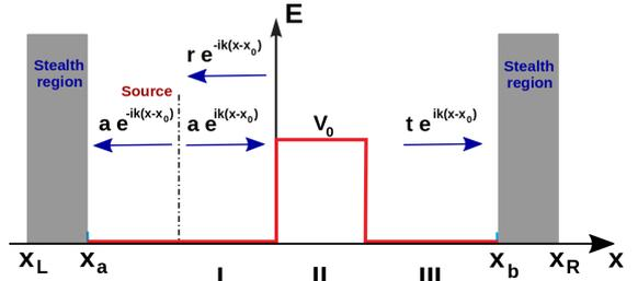
Fig. 2: Scattering through a 1D barrier of height  $V_0$  with stealth region on either side of the barrier. We consider a source at  $x = x_0$  within the active region which injects an incoming wave with an amplitude  $a$  and the energy  $E$  in both directions. The corresponding wavevector is  $k = \sqrt{2m^*E/\hbar^2}$ . Here,  $r$  and  $t$  are the reflection and transmission coefficients respectively.
