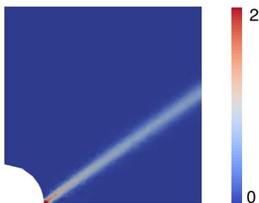
Fig. 3 Distribution of magnitude of strain rate (873 elements)
