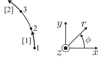
Fig. 2 Line element with 2-edges and 3-nodes
