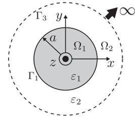
Fig. 3 Cross section of a cylindrical dielectric waveguide
