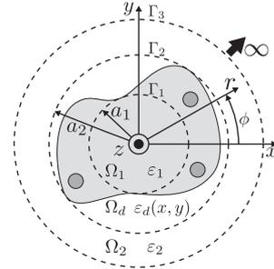
Fig. 1 Cross section of a dielectric waveguide
